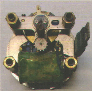
Above: Clock internal with body removed and solenoid still in position.
