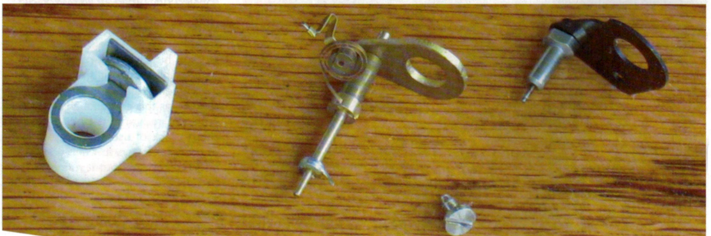
The failed contacts and associated fittings – the weak link in the original Smiths clock. These are the parts replaced by the Clocks4Classics PCB board. Keep them if you ever wish to return to the original Smiths timepiece.
