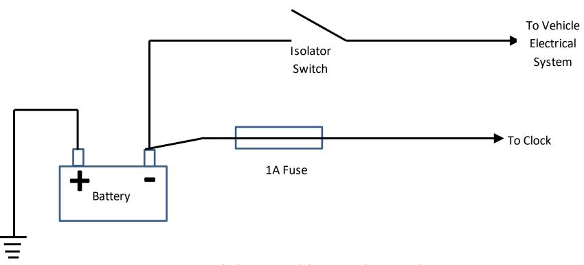
Clock wiring with battery isolator switch
